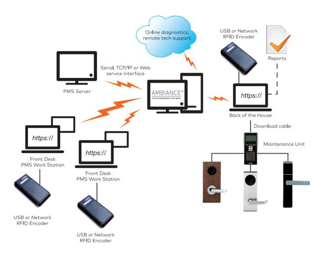
\* Network RFID encoders communicate directly to the server and require an open port on the server to connect.
